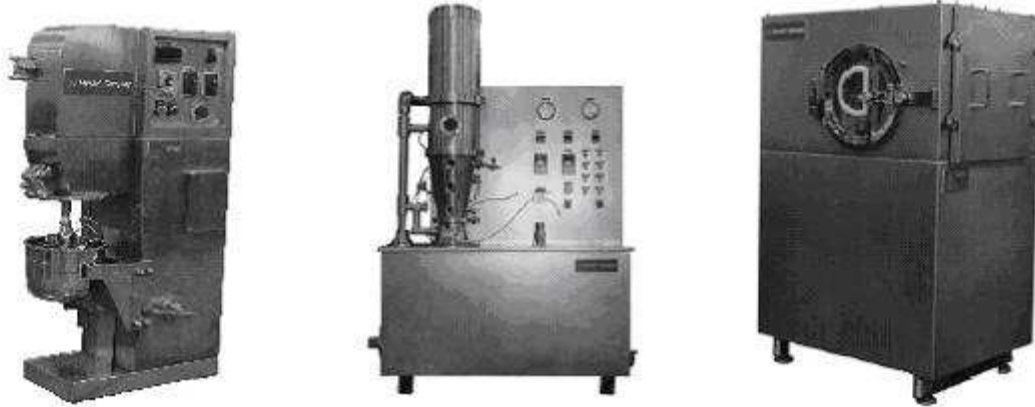
Laboratory High Shear Mixer, Fluid Bed Processor and Perforated Pan Tablet Coater
